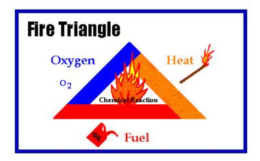
Extinguishing a fire is achieved by removing any element of the three sides of the triangle.
